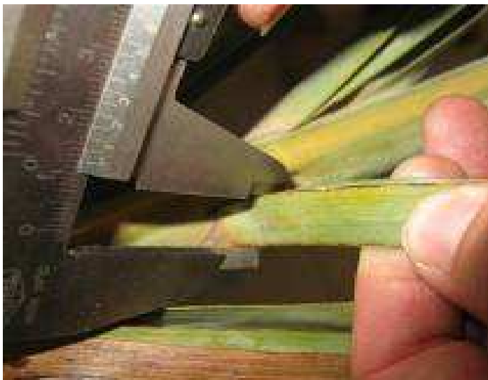
3.7.2 Measurement of half-width, at the position 1/3 of length, using a graduate strip or a metal tape measure
