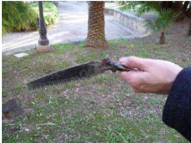
Fig.5. zirconium-steel blade used with the carbon fiber pole Fig.6. Elevator
