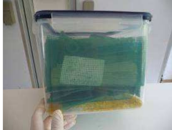
Fig.14 and 15. Airtight box containing dried leaf samples and, on the bottom, some silica gel
